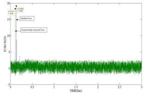
Fig.4. Comparison of Identified force at 2 with the measured force in time domain
