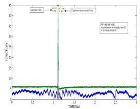
Fig.7 Comparison of Identified force at 5 using FRF  $[H_{45} H_{65} H_{105}]$  T with the measured force
